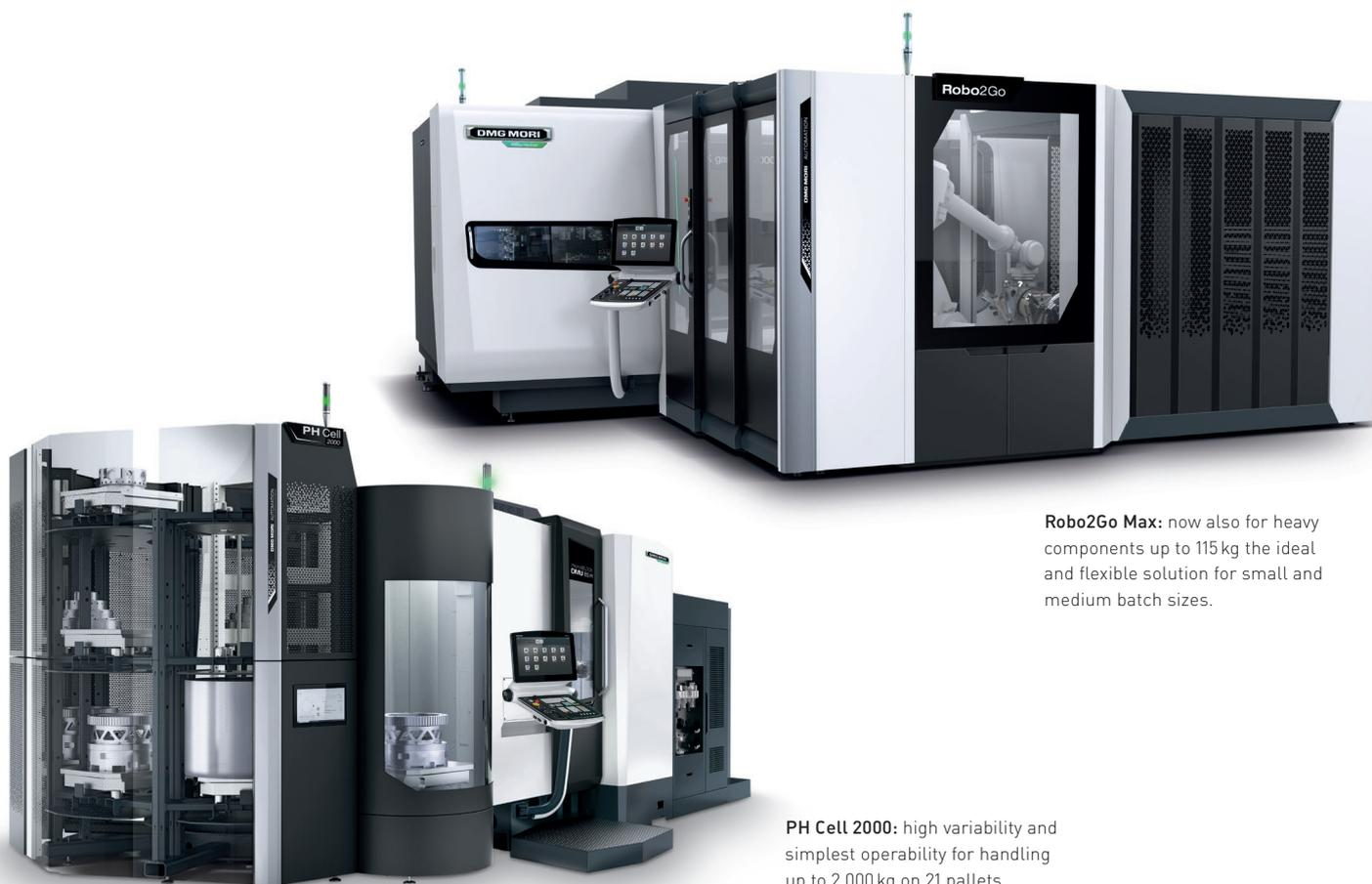
**Robo2Go Max:** now also for heavy components up to 115 kg the ideal and flexible solution for small and medium batch sizes.
